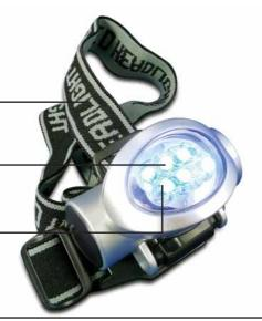
The LED headlamp is ideal to use on-site where ambient light is poor or absent. It is lightweight and comfortable to wear thanks to its elastic band. LEDs emit white light with three selectable levels of intensity, offering longer life than traditional incandescent bulbs while consuming less power, increasing its battery life. It works with 3 AAA batteries.
