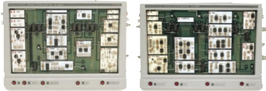
The analogue communications training system **EC-696** has several types of emitters, transmission channels, receivers, modulators and demodulators, in order to shape a transmission system easily. For instance, it permits to compare the advantages of several transmission systems to others, including those fibre-optics based, or to analyse interference phenomena.
