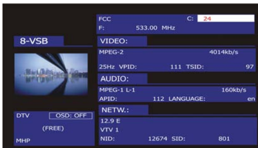
Figure 60.- Digital channel monitoring.
