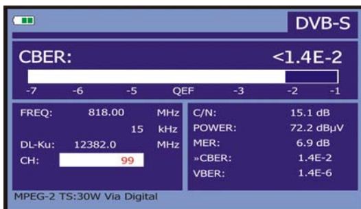
Figure 38.- DVB-S (QPSK) signals CBER measurement screen.
