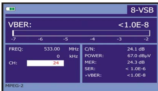
Figure 36.- Screen of BER measurement 8-VSB signals. VBER
