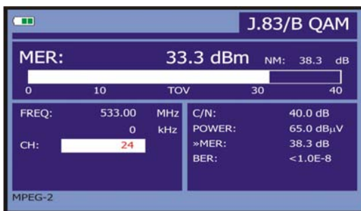
Figure 31.- Screen of BER measurement of QAM Annex-B signals.
