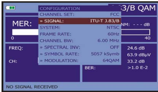
Figure 20.- Screen of measurement configuration ( QAM Annex-B signals).
