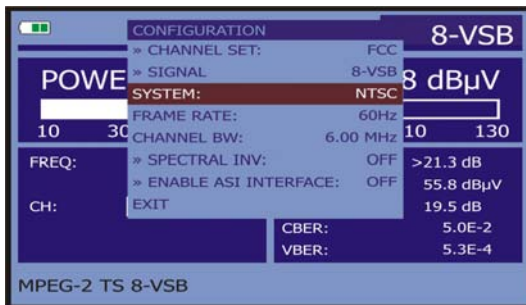
Figure 21.- Screen of measurements configuration ( 8-VSB signals).
