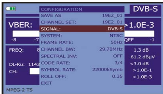
Figure 22.- Measurement configuration screen (QPSK signals).
