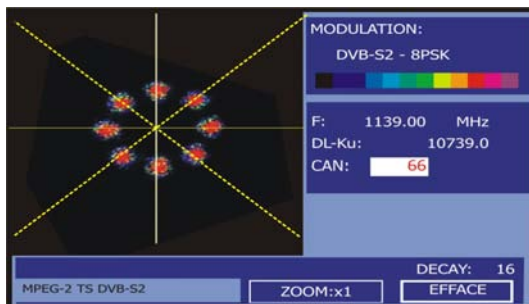
Figure 49.- Diagramme de constellation. Signal DVB-S2 (8PSK).
