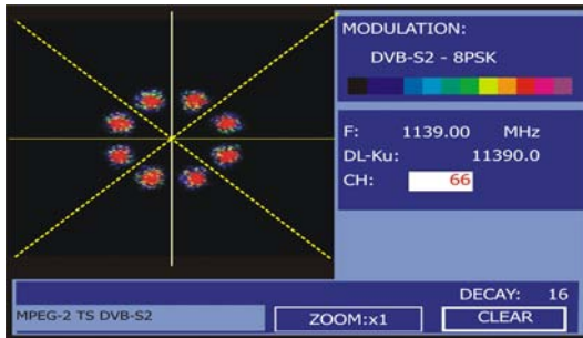
Figure 49.- Constellation Diagram. DVB-S2 (8PSK) signal.
