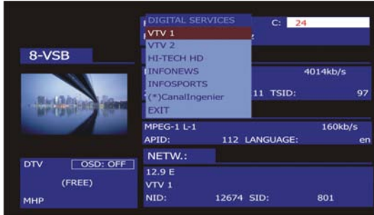
Figure 61.- Digital channel monitoring. Digital services.
