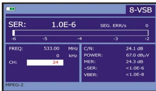
Figure 37.- Screen of SER measurement ( 8-VSB signals).
