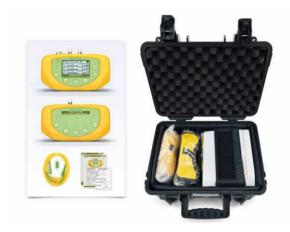
Simplify fiber cabling certification in buildings with this device. It enables a single operator to certify all optical outlets by connecting the **PROLITE-105** light source to the building's fiber optic input, automatically generating pilot signals. The operator then uses the **PROLITE-67** FTTH meter to verify the received optical power at each outlet.
