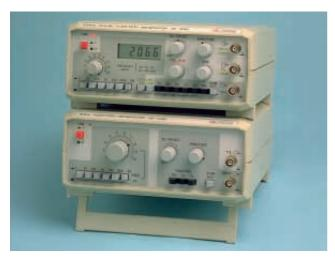
The GF-230 is a function generator covering the frequency range from 0.1Hz to 1MHz in seven decades. It allows to generate sinusoidal, square and triangular waves with continuous control of the output level, fixed 20 attenuator and the possibility to superimpose the signal at a continuous level through the DC OFFSET control. The VCO input located on the rear panel enables the user to control the output frequency and performs FM modulations to any auxiliary signal.
