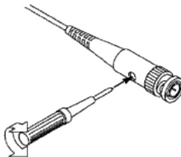
Figure 8. Adjust Probe.
