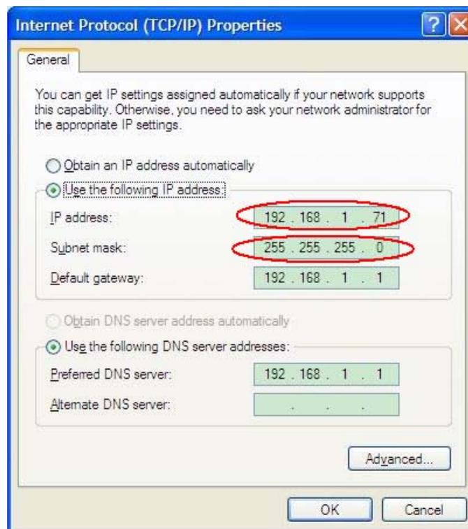
Figure 74. Set the network parameters of the computer.
