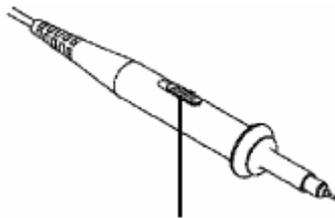
Figure 9. Attenuation Switch.
