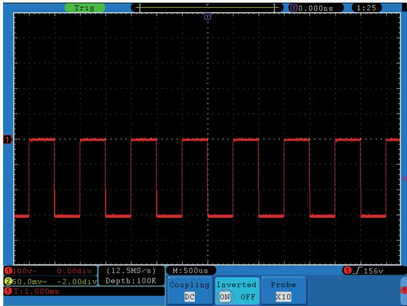
Figure 18. Inverted Waveform.
