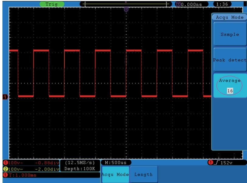
Figure 84. Reduce Noise level by using Average function.
