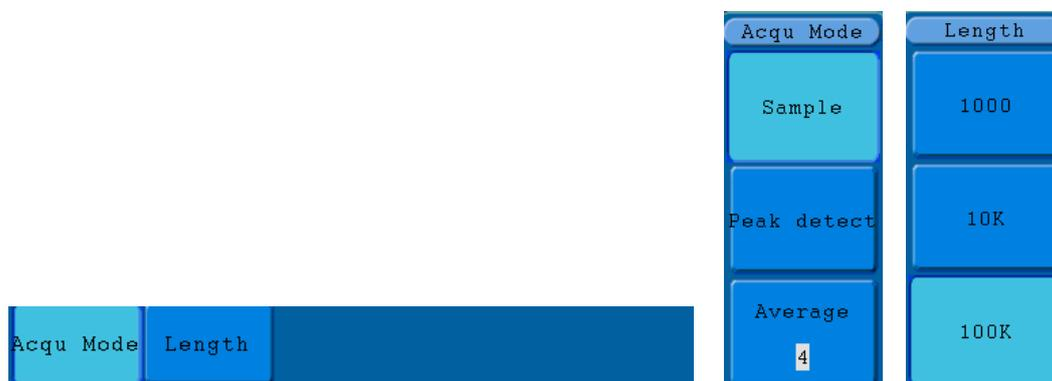
Figure 38. ACQU MODE Menu (OD-603 does not have "Length" menu).
