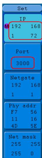
Figure 76. Set the network parameters of the oscilloscope.
