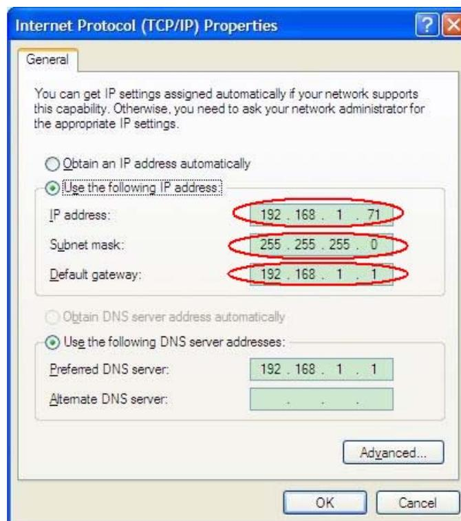
Figure 77. Set the network parameters of the computer.
