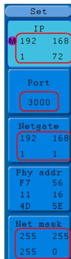
Figure 79. Set the network parameters of the oscilloscope.
