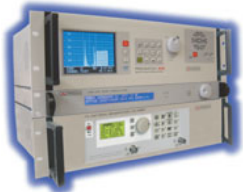
DTT complete test set using GV-998 as an encoder
