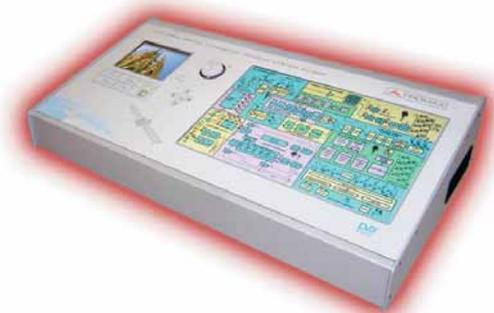
Thanks to the possibility of **DVB-T signals broadcasting** through an antenna it is possible to simulate a real broadcast transmission. Moreover, using an additional antenna it makes possible the analysis of the DVB-T signal including every parameter involved, in such way that the student is able to understand the pros and cons of the different configurations.
