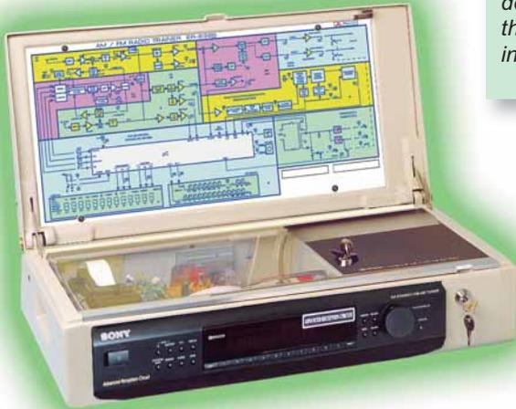
The **ER-832 Radio Training System** is an educational instrument designed for the theoretical/practical study of the operation of the advanced radio receivers through analysis of the main signals involved in different processes.
