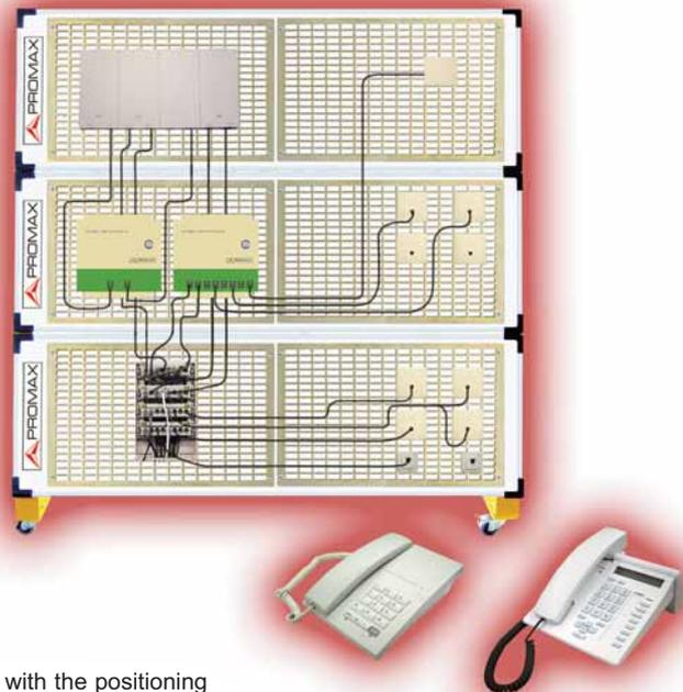
Each one of the **ET-836** modules has an active block diagram, with telephone connectors and test points, that allow the connexion of telephone lines and the terminals. In the test points the telephone signals can be observed, to analyse their different states and to measure their parameters. Also they allow the study of the typical errors of wiring.
