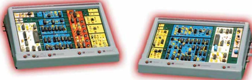
The **emitter** and **receiver** modules have a number of test points prepared for the monitoring of the signals. The **EC-796** allows the development of experiments at five levels:
