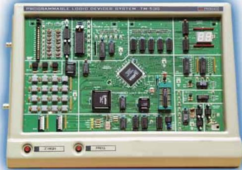
The **TM-530** trainer is an innovative educational tool specifically created for easily learning the design, programming and development of applications using programmable logic devices (PLD). It may also be used professionally as an agile testing instrument for designing logic circuits without the need of creating connections or welding, or wasting time building circuits. The instrument consists of:
