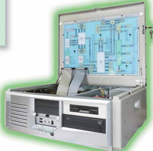
The trainer includes a powerful latest-generation **multimedia PC**, **Intel® Core™ 2 Duo** processor, a **breakdown module** and an **active block diagram** which allows to analyse the main signals of the PC hardware, as well as its peripherals. The training system also includes a **15" Multimedia monitor**.
