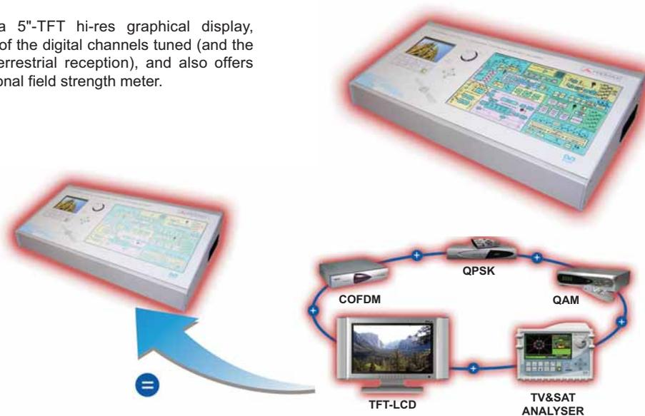
In the aspect of measures, highlights the spectrum dynamic exploration to detect all the transmissions existing in the explored band, the measurement of power level, the carrier/noise ratio (C/N), the digital signal error rate (BER) and the modulation error ratio (MER), as much for DVB-T (COFDM) signals as DVB-S (QPSK) and DVB-C (QAM) signals.
